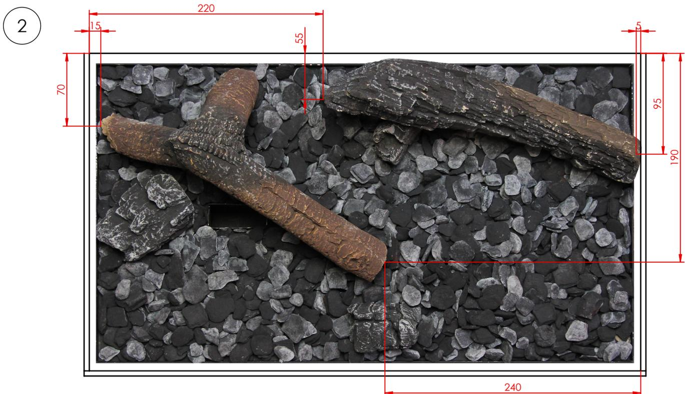
**EN** **Log set 05:** Chips have to be placed as shown. The black and grey chips have to be mixed before spreading them evenly. Beware to keep the pilot free at all times and make sure that there is no fine dust on the burner. Place the logs exactly as shown on the figure. The enclosed amount must be strictly respected.
